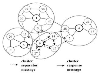
Figure 8. Settlement of spreading code and TDMA schedule
