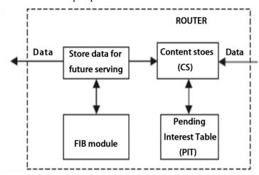
Figure 1. Named Data Network Architecture
