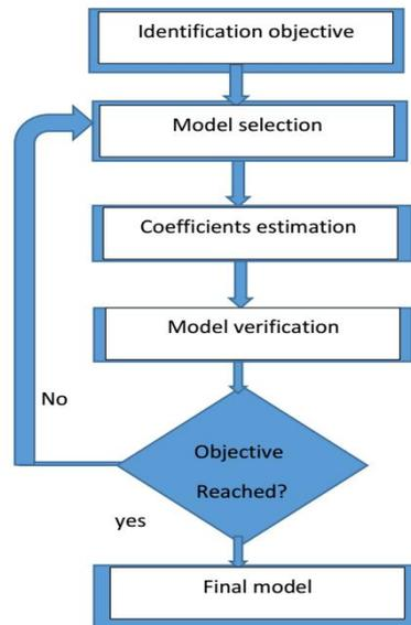
Figure 3. Architecture Diagram of System Identification
