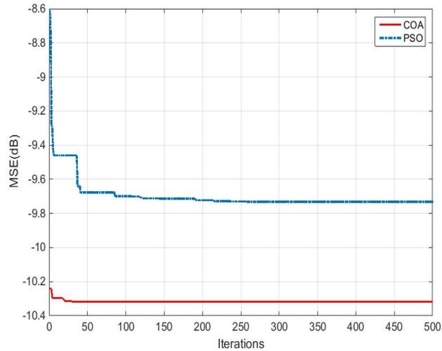
Figure 10. Convergence Curves of a Volterra System Identification Given in Example 6
