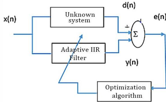
Figure 1. The graphical representation of the Identification Process
