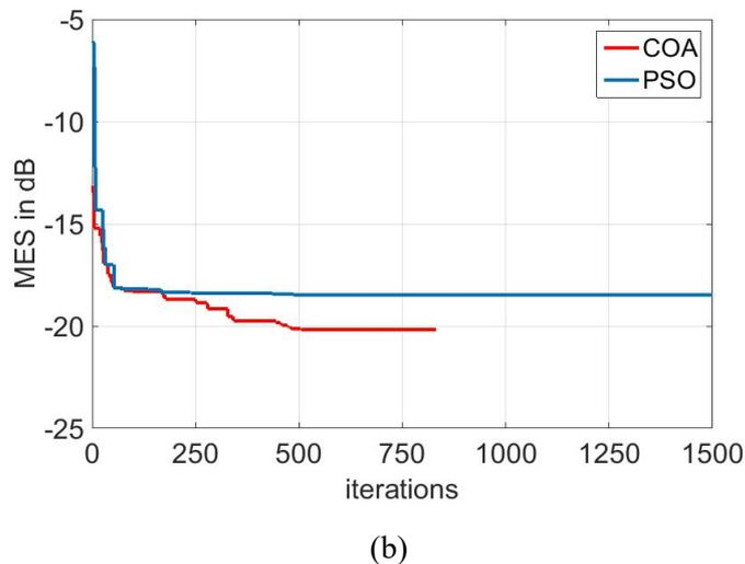
Figure 6. Convergence Curves for a 3<sup>rd</sup>-order System Identified by (a) 3<sup>rd</sup>-order Filter and (b) 2<sup>nd</sup>-order Filter
