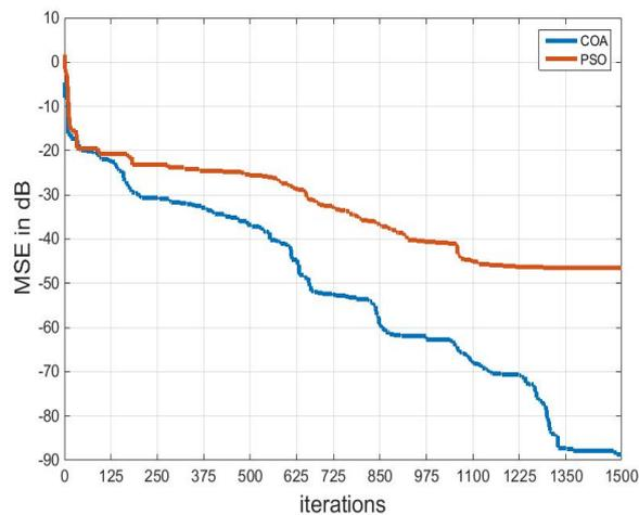
Figure 4. Convergence Curves for 4th-order Filter Representing 4th-order System
