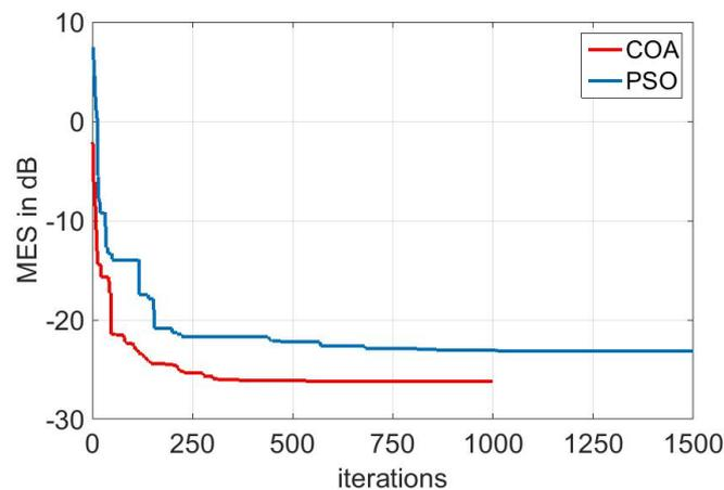
Figure 7. Convergence Curves for 3<sup>rd</sup>-order System Identified by (a) 3<sup>rd</sup>-order Filter (b) 2<sup>nd</sup>-order Filter
