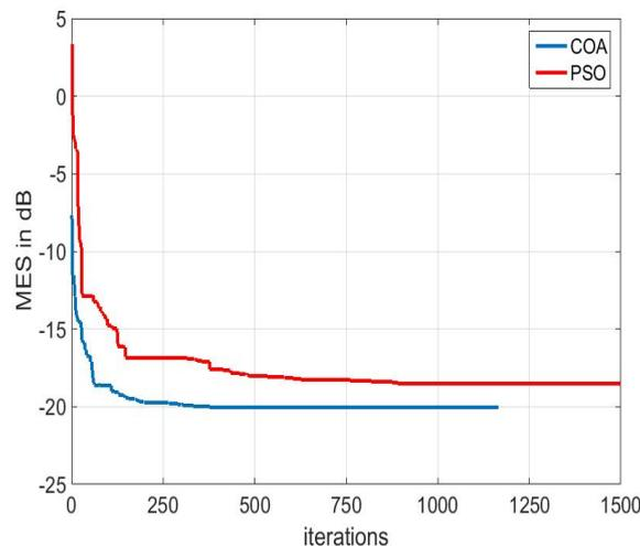
Figure 5. Convergence Curves for 3<sup>rd</sup>-order Filter Representing 4<sup>th</sup>-order System
