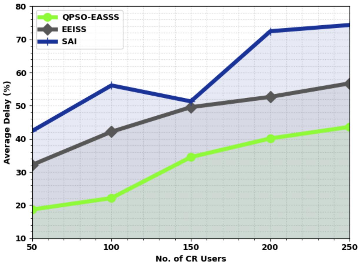
*Fig. 7. ADEL analysis of QPSO-EASSS system with varying CR users*
