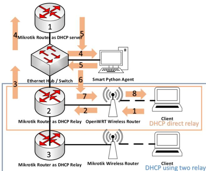
Figure 5. Smart Agent and DHCP relay in default Mikrotik Scenario
