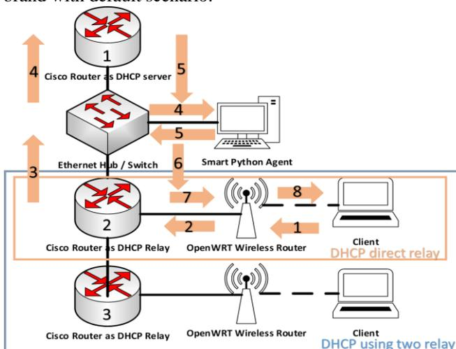
Figure 1. Smart Agent and DHCP relay in default Cisco Scenario
