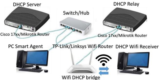
Figure 7. Real network devices and interfaces involved in the research scenarios
