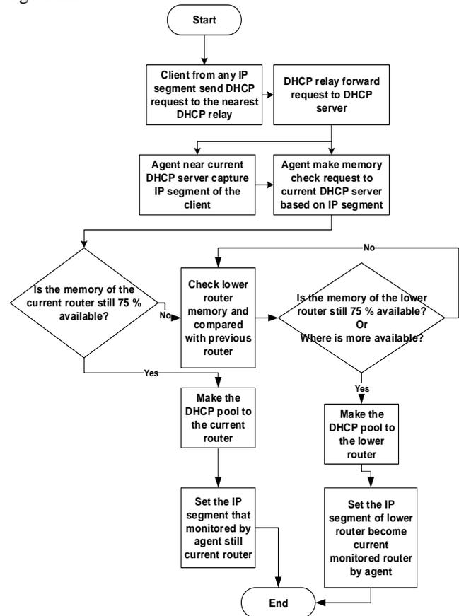
Figure 8. DHCP modified master-backup selection algorithm
