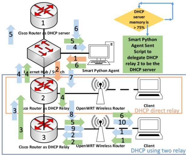
Figure 4. Smart Agent and DHCP relay using Smart Agent Cisco Scenario when DHCP relay take over the DHCP server duty
