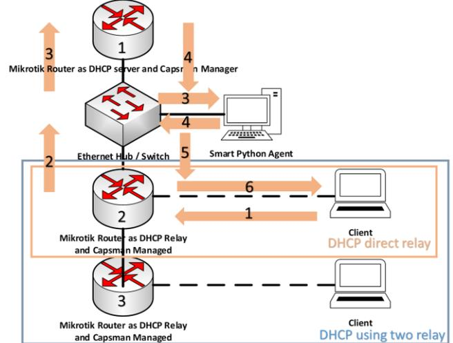
Figure 6. Smart Agent and DHCP relay in default Mikrotik Scenario with “Capsman” protocol
