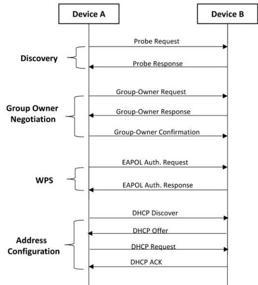
Figure 3. Communication protocol with Wi-Fi Direct.
