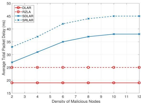
**Figure 10.** Effect of malicious nodes on average total packet delays for 40 vehicular nodes and 5 units/sec node speed.
