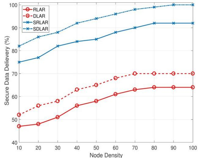
Figure 7. Effect of node density on secure data delivery for 10% malicious nodes and 5 units/sec node speed.
