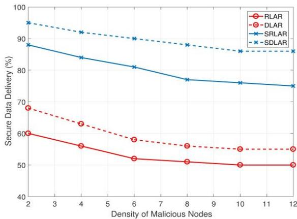
**Figure 9.** Effect of malicious nodes on secure data delivery for 40 vehicular nodes and 5 units/sec node speed.
