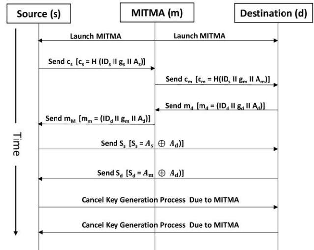
Figure 6. Discovery of the man-in-the-middle attack (MITMA) security threat.
