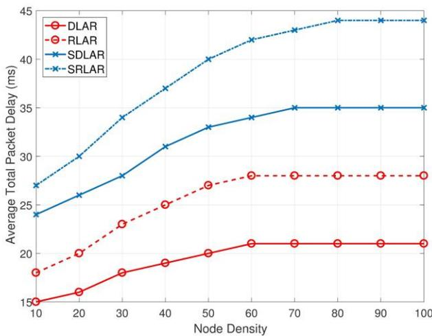
**Figure 8.** Effect of node density on average total packet delay for 10% malicious nodes and 5 units/sec node speed.
