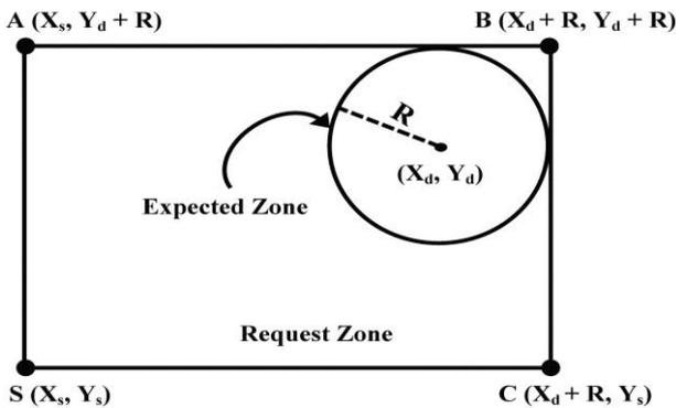
**Figure 1.** Request zone when  $\text{Dist} > R$ . Source node S is out of the expected zone of destination node D.
