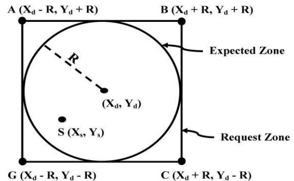
**Figure 2.** Request zone when  $\text{Dist} \leq R$ . Source node S is in the expected zone of destination node D.
