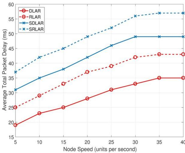
**Figure 12.** Effect of node speed on average total packet delay for 40 vehicular nodes and 10% malicious nodes.
