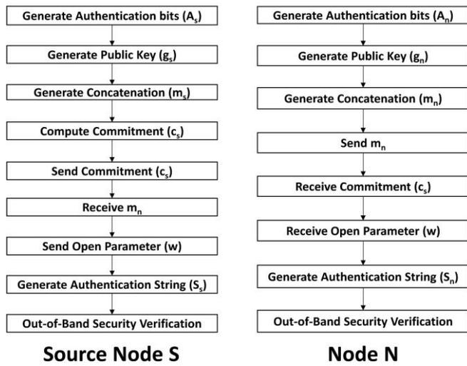
**Figure 4.** Security authentication model at source node S and node N.
