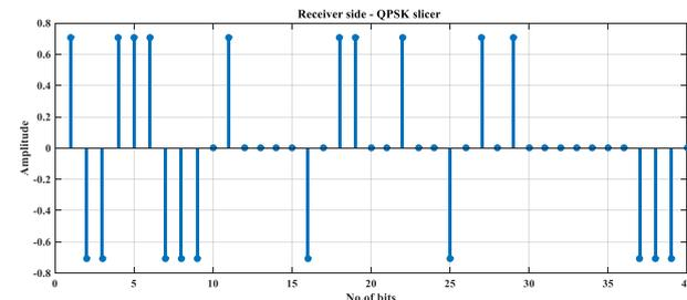
**Figure 10.**Received bits across a noisy channel
