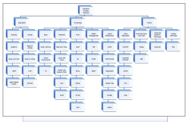
Figure 4: Routing Protocols of OPPNETS- Replication, Forwarding and Hybrid
