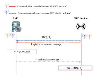
Figure 2. The registration phase in SAP-NFC protocol
