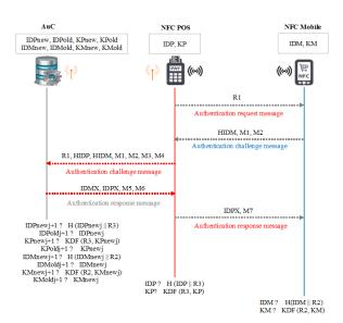
Figure 3. The authentication phase in SAP-NFC protocol
