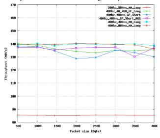
Figure 5. Throughput versus the packet sizes for varying parameters combinations using TCP protocol
