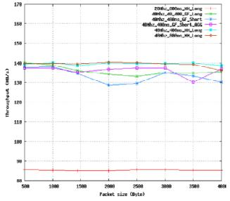
Figure 4. Throughput versus the packet sizes for varying parameters combinations using UDP protocol
