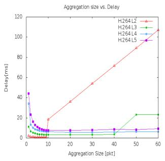
Figure 11. Average delay versus the aggregation size for video applications
