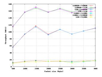
Figure 6. 802.11n interoperability and coexistence for various operating mode
