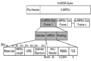
Figure 2. A-MPDU frame format
