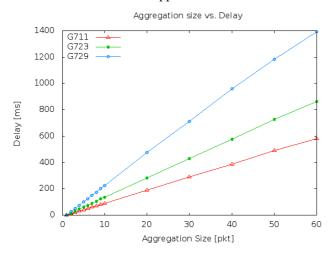
Figure 9. Average delay versus the aggregation size for voice applications
