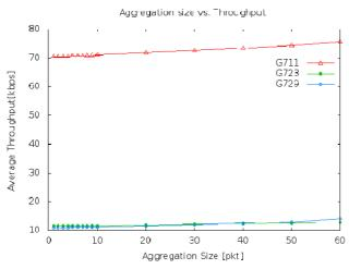
Figure 8. Average throughput versus the aggregation size for voice applications
