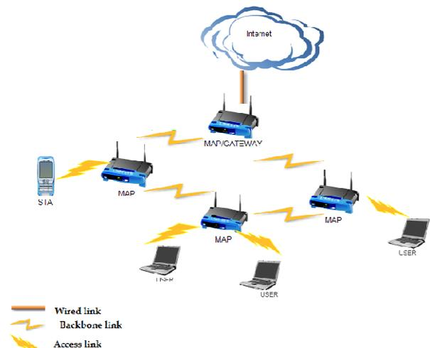
**Figure 1** Wireless mesh network architecture
