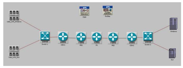
Figure 4. OPNET Network Setup
