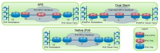
Figure 3. 6PE, Dual Stack, and Native IPv6 Transition Mechanisms
