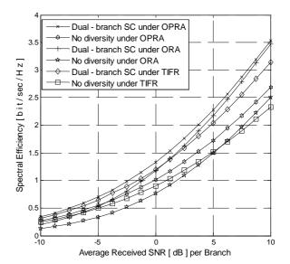
Figure 5. Spectral Efficiency versus average received SNR  $\bar{\gamma}$  under different adaptive transmission schemes.
