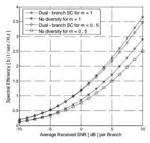
Figure 2. Spectral Efficiency versus average received SNR  $\overline{\gamma}$  under ORA.
