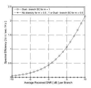
Figure 4. Spectral Efficiency versus average received SNR  $\bar{\gamma}$  under CIFR.
