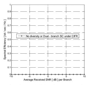
Figure 3. Spectral Efficiency for a worst-case of fading versus average received SNR  $\overline{\gamma}$ .
