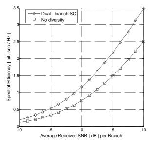
Figure 1. Spectral Efficiency for a worst case of fading versus average received SNR  $\overline{\gamma}$  under ORA.
