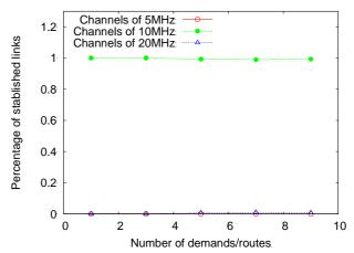
Figure 14. Percentage of established links while selecting channel width for B-MTM metric
