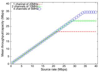
Figure 4. Throughput and capacity of 1, 2 and 4 orthogonal channels of 20, 10 and 5MHz. (CBR source)
