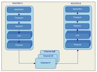
Figure 3. Routers transmitting in multiple orthogonal channels.
