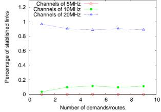
Figure 10. Percentage of established links in each channel width for WCETT metric
