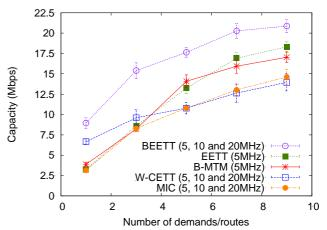
Figure 20. Greater obtained capacity values by selecting or using individual channel widths of 5, 10 and 20MHz)
