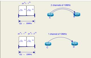
Figure 2. Spectrum division into physical (group of channels) and individual channels
