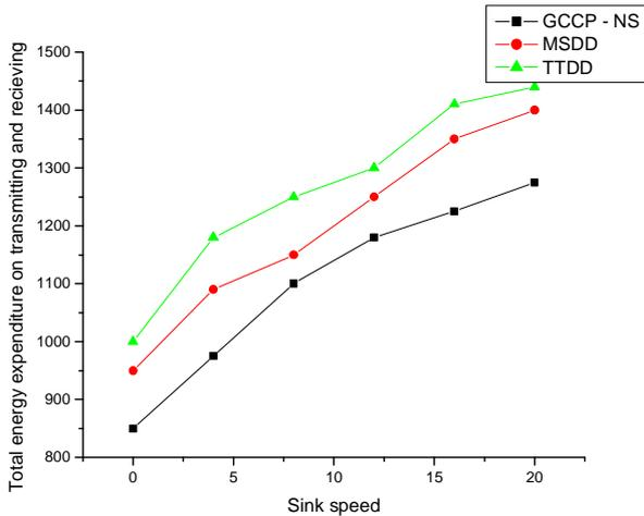
Figure 6. Energy expenditure with respect to Sink speed
