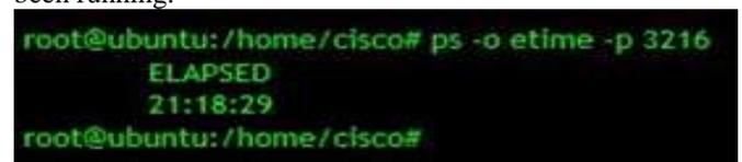
**Figure 23: Output of the ps command for PID 3216.**
