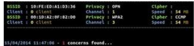
**Figure 30:** Output of wids.py upon detecting a potentially malicious access point.
