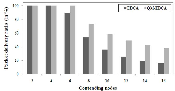
**Figure 10.** Packet delivery ratio vs. density/Traffic-load for EDCA and QM-EDCA
