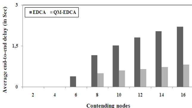
**Figure 8.** Average end-to-end delay vs. Density/Traffic-load for EDCA and QM-EDCA
