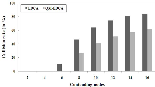
**Figure 7.** Collision rate vs. Density/Traffic-load for EDCA and QM-EDCA
