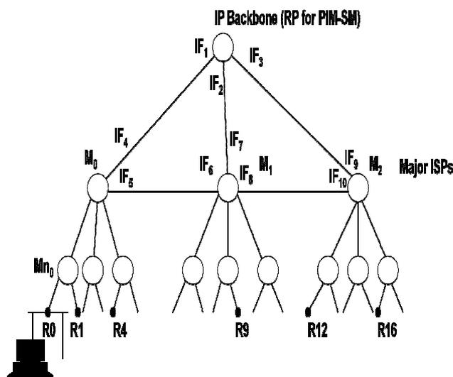
Figure 1. Non-strictly hierarchical network architecture. Note that  $R_0$  serves as designated router (DR) and root of the data source, leaf routers  $R_1$ ,  $R_4$ ,  $R_9$ ,  $R_{12}$  and  $R_{16}$  are active members of the group. **IF** refers to interface.
