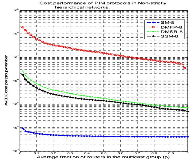
Fig. 4: Performance of the PIM protocols when minor ISPs are connected.
