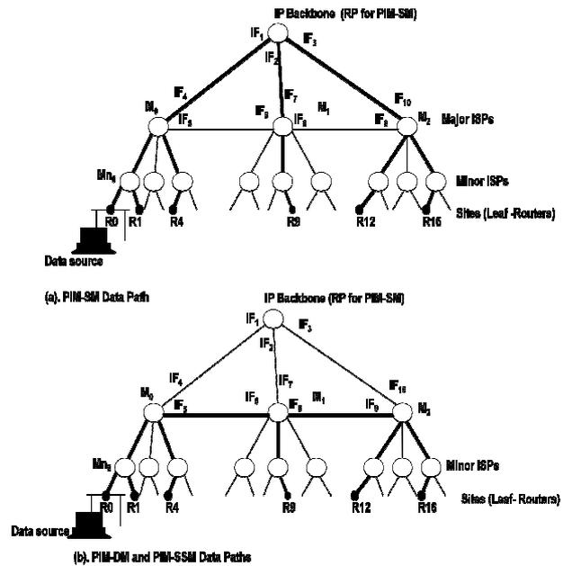
Figure 2. (a) The thick links show the distribution data path of the PIM-SM protocol, (b) the thick links show the data paths of the PIM-DM and PIM-SSM protocols.
