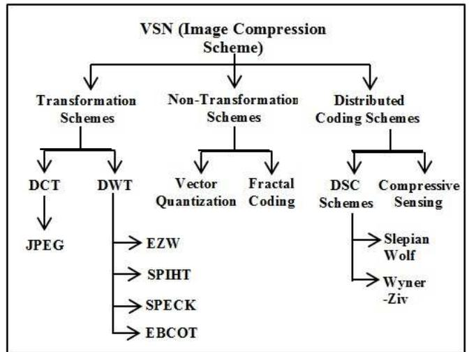
Figure 3. Classification of image compression scheme for VSN
