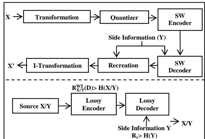
**Figure 5.** Overall block diagram of WZ encoder along with lossy decoder
