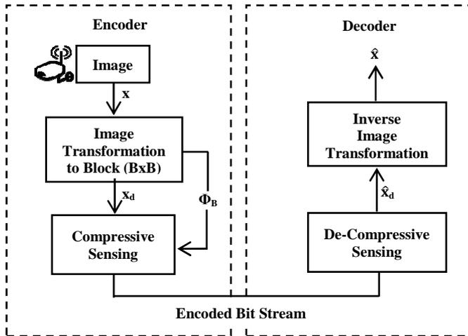
**Figure 6.** Broad spectrum block diagram of Image compression and decompression by using compressive sensing scheme.
