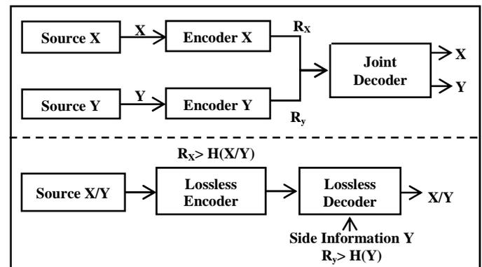
**Figure 4.** General Structure of SW algorithm along with lossless decoder
