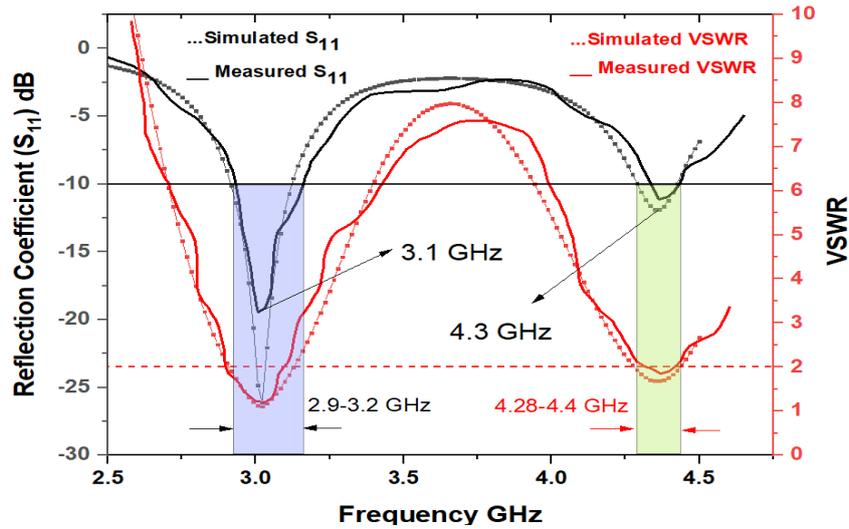
Figure 4. Reflection Coefficient & VSWR Vs Frequency
