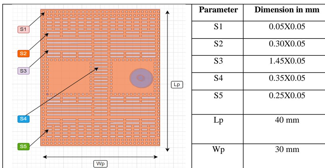
**Figure 2.** Fractal Antenna Structure
