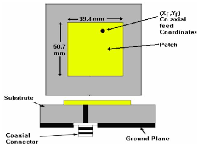
Figure 1. Coaxial fed micro strip patch antenna
