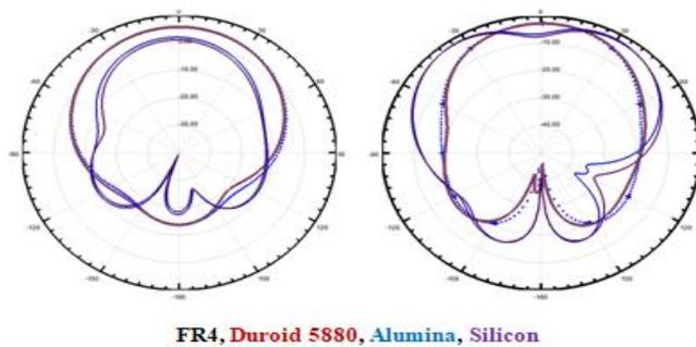
**Figure 11.** Radiation pattern variation with change in substrate material
