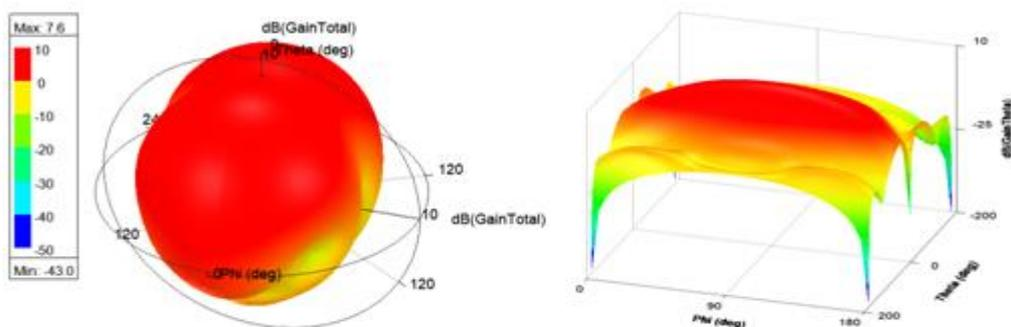
Figure 6. 3D-Gain at 4.3 GHz
