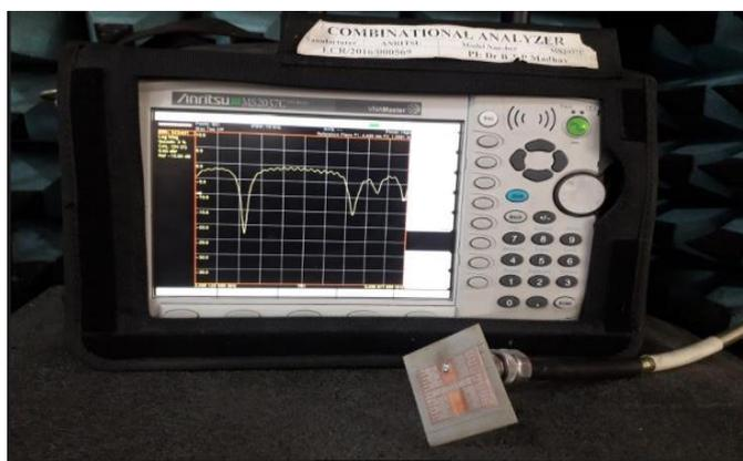
**Figure 9.** Measurement of  $S_{11}$  on Anritsu VNA
