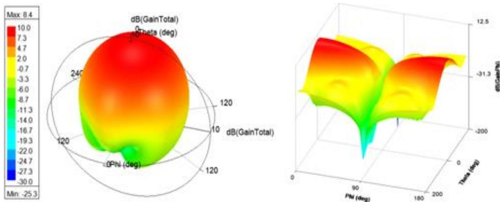
Figure 5. 3D-Gain at 3.1 GHz
