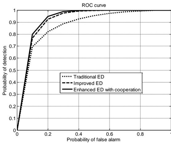
Figure 5. ROC curves for SNR = -10.87 dB
