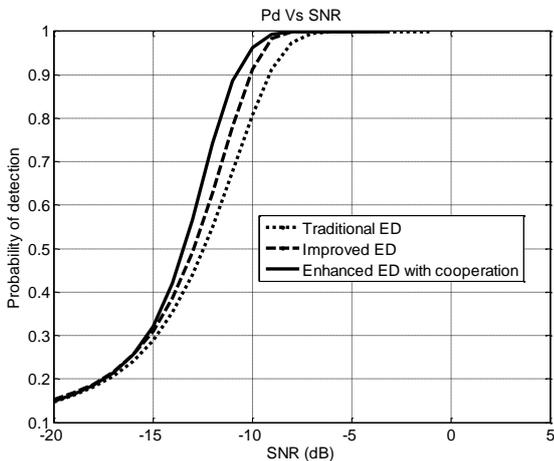
Figure 11. Performance comparison of the algorithms with respect to SNR
