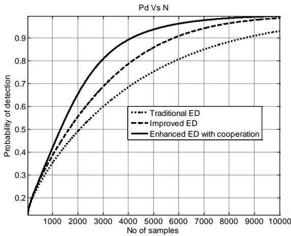
**Figure 13.** Performance comparison of the algorithms with respect to the number of samples
