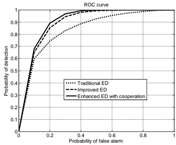
Figure 6. ROC curves for SNR = -11.61 dB
