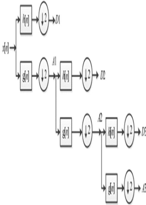
Figure 3. Signal Decomposition into Sub-bands
