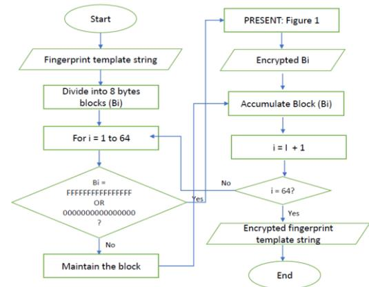
Figure 7. The flow chart of header and zero blocks bypass method
