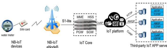
**Figure 3.** Network architecture of NB-IoT network for water meter application
