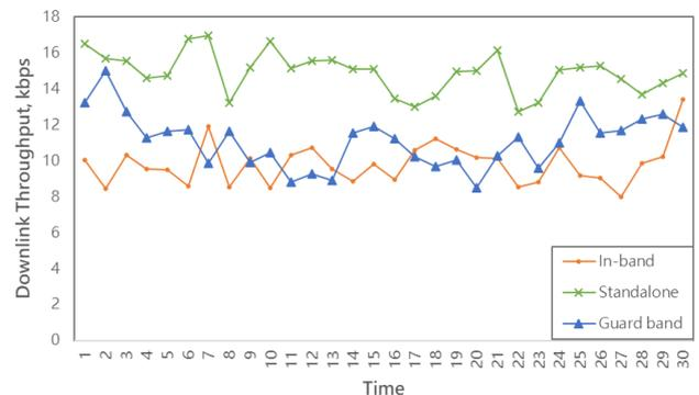
**Figure 5.** Measurements of Downlink Throughput in Busy Hour (BH) during period of 30 days
