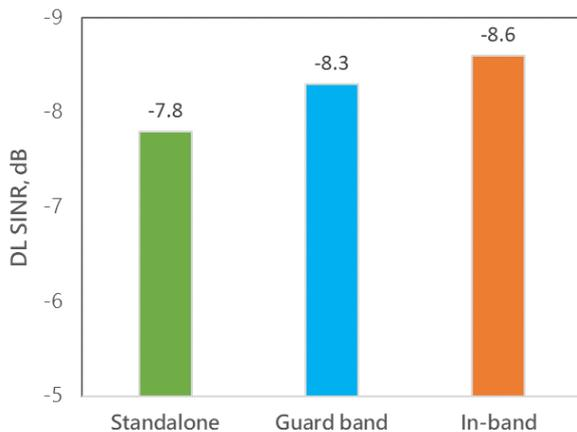
**Figure 4.** Downlink SINR measurements for different NB-IoT deployment modes
