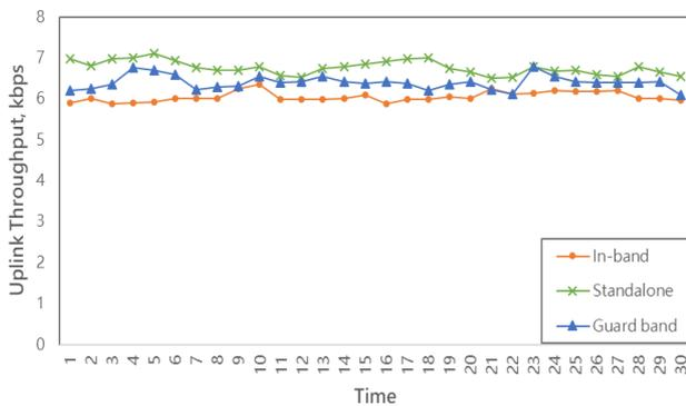
Figure 6. Measurements of Uplink Throughput in Busy Hour (BH) during period of 30 days
