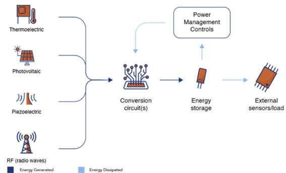
**Figure 1.** Energy harvesting flow of IoT devices
