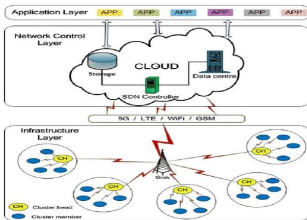
Figure 2. Cluster based energy harvesting IoT network
