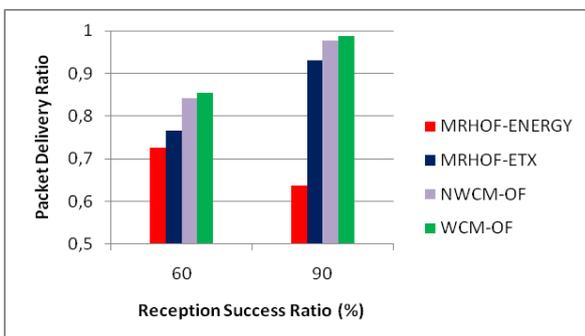
**Figure 4.** Performances in term of packet delivery ratio for 20 nodes.
