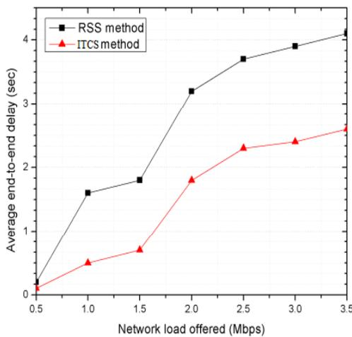
Figure 9: Network load vs E2E delay
