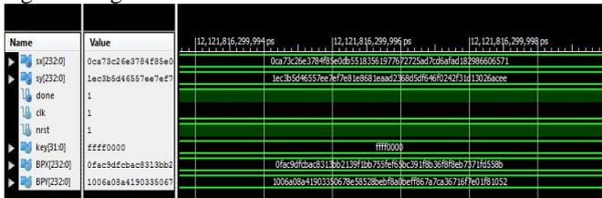
Figure 14. Simulation result of scalar multiplier using karatsuba multiplier.
