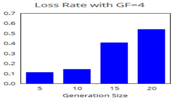
Figure 7. Packet Loss Vs. Generations (GF=4)
