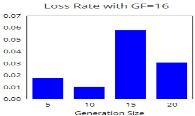
Figure 9. Packet Loss Vs. Generations (GF=16)
