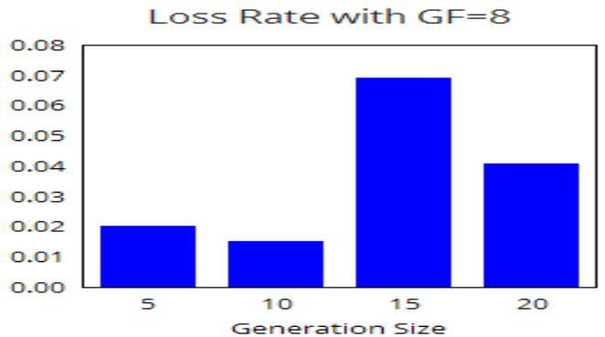
Figure 8. Packet Loss Vs. Generations (GF=8)
