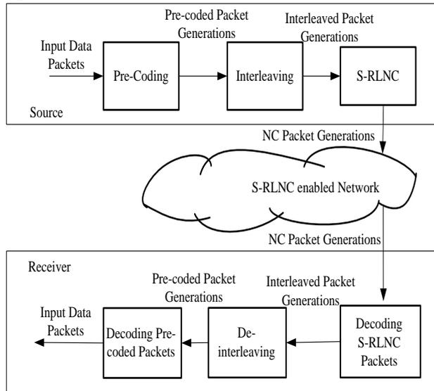
**Figure 1.** Block diagram of Pre-Coding and Interleaving assisted S-RLNC for MBMS
