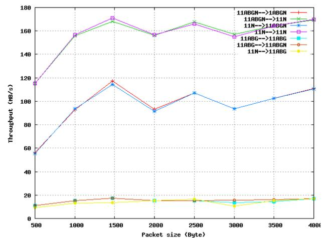
**Figure 6.** 802.11n interoperability and coexistence for various operating mode
