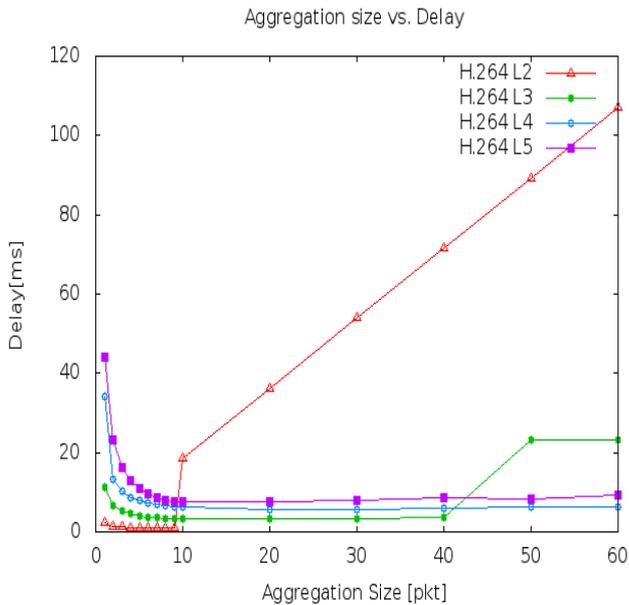
Figure 11. Average delay versus the aggregation size for video applications
