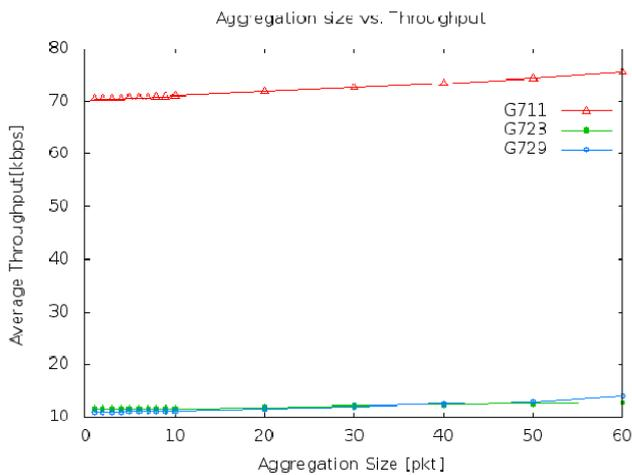
**Figure 8.** Average throughput versus the aggregation size for voice applications
