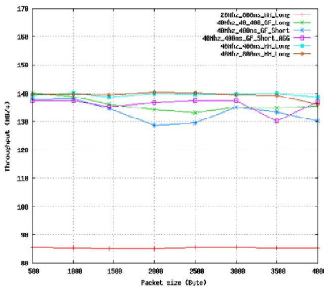
**Figure 4.** Throughput versus the packet sizes for varying parameters combinations using UDP protocol
