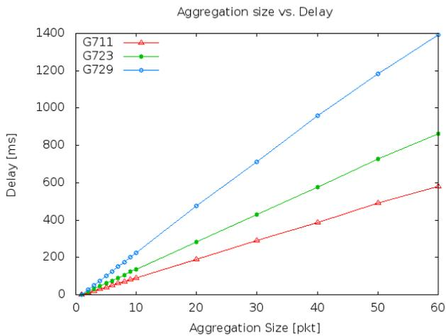
**Figure 9.** Average delay versus the aggregation size for voice applications
