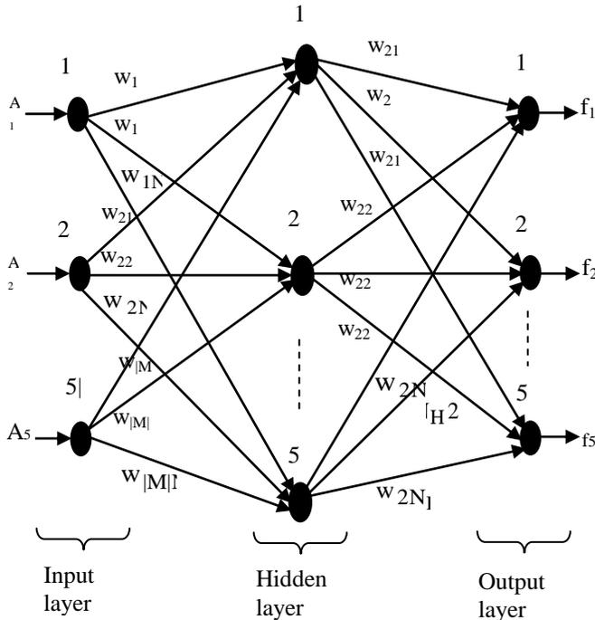
**Figure 3:** Structure of FFBNN classifier i.e. Neural Network hidden layer
