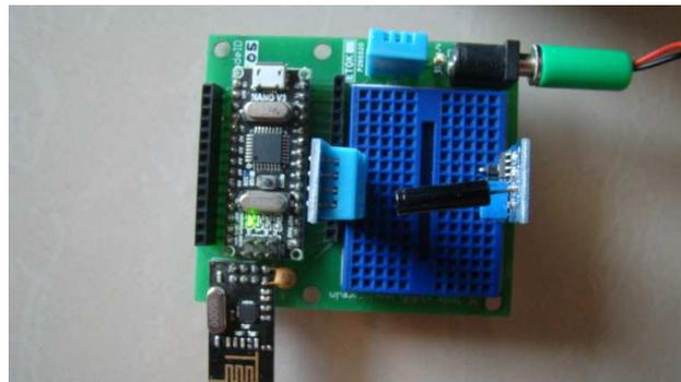
**Figure 7.** Top view of physical view of RF node which is used for experimentation
