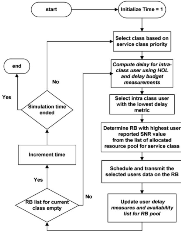
Figure 14. Delay Based Scheduling step [4]
