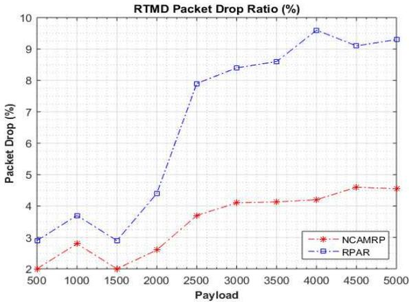
Figure 5. RTMD Packet Drop ratio with payload variation
