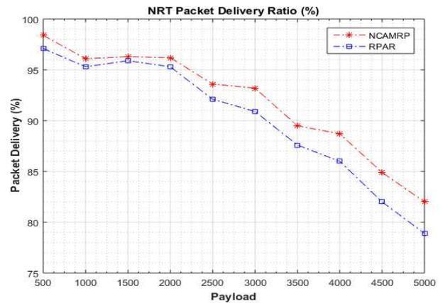
**Figure 4.** Non-real time multimedia data (NRT) delivery with payload variation
