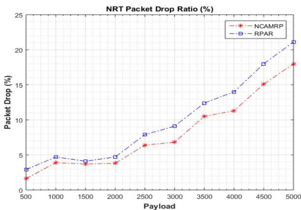
Figure 6. NRT Packet Drop ratio with payload variation
