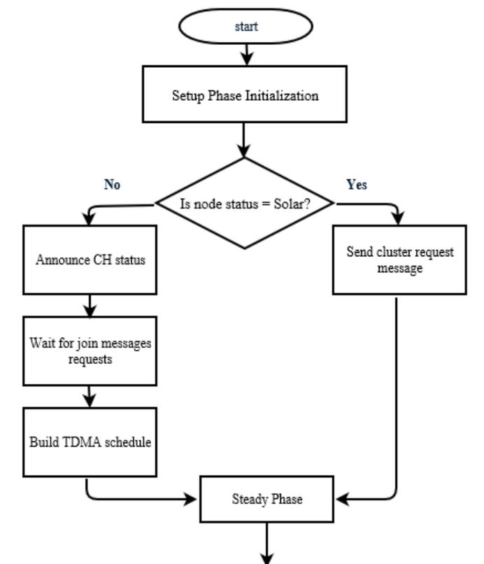
Figure 1. The process of selecting CHs
