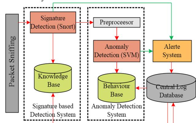
Figure 2. Architecture of C-NIDS framework proposed
