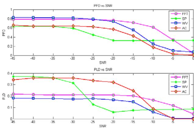
Figure 7. PFD and PLD vs. SNR (OFDM)
