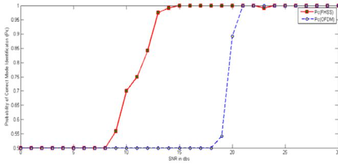
**Figure 9.** Probabilities of correct mode Identification for FHSS and OFDM
