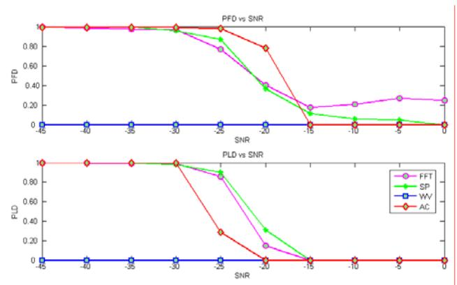
Figure 5. PFD and PLD vs. SNR for FHSS signal
