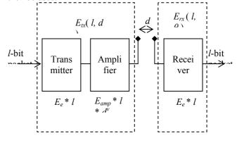
Figure 3.1: Radio Energy Consumption Model in LEACH-IMP
